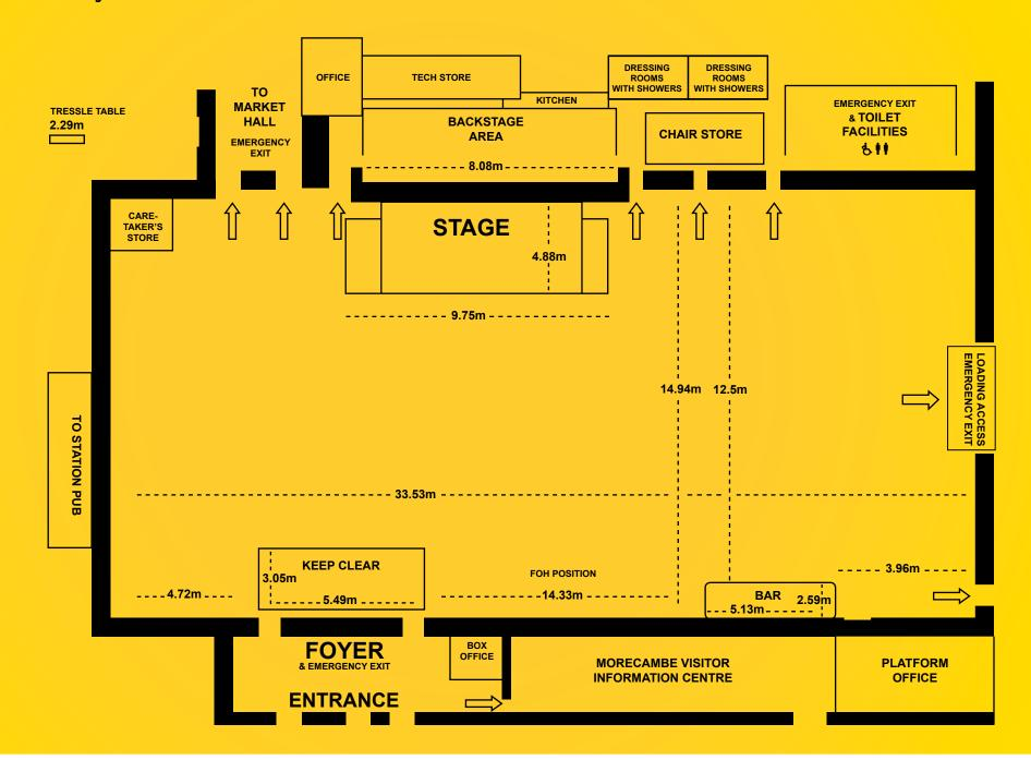
**The Tech Spec** - The main performance space is an open area of 37.3m x 15m with a quality Granwood flooring system and a modular steel deck thrust stage in the centre. The stage can be tailored to requirements in terms of position, height, size and shape but regularly stands at 9.7m x 4.8m with black drapes as a backdrop.
