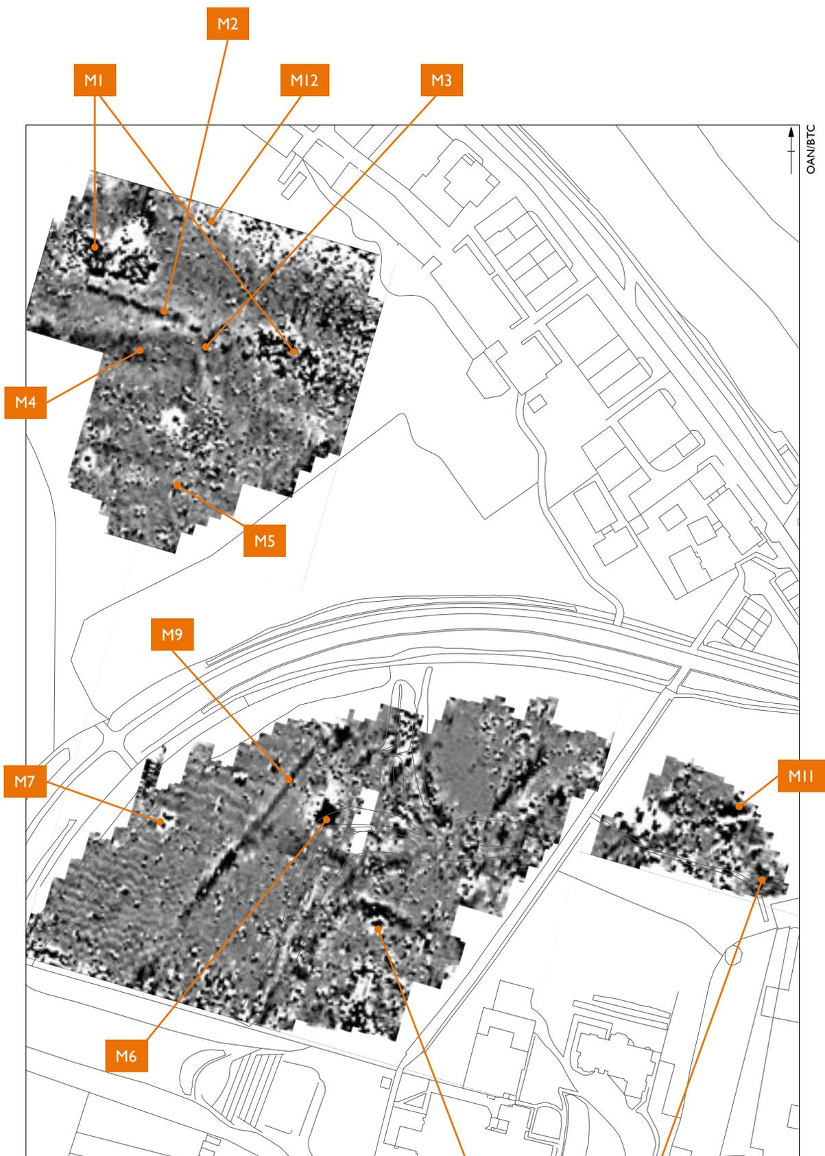
*Magnetometry survey of Vicarage Field West and East and Quay Meadow. For ease of reference the numbering of the anomalies follows that used in the OAN report with the addition of M12*
