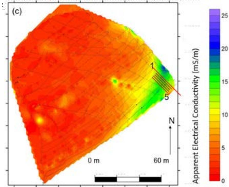
EMI survey of Quay Meadow showing the anomaly at the eastern edge of the survey area and position of the 2D-ERT sections
