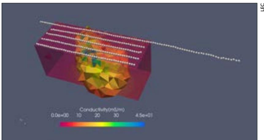
3D-ERT model of the suspected tidal inlet
