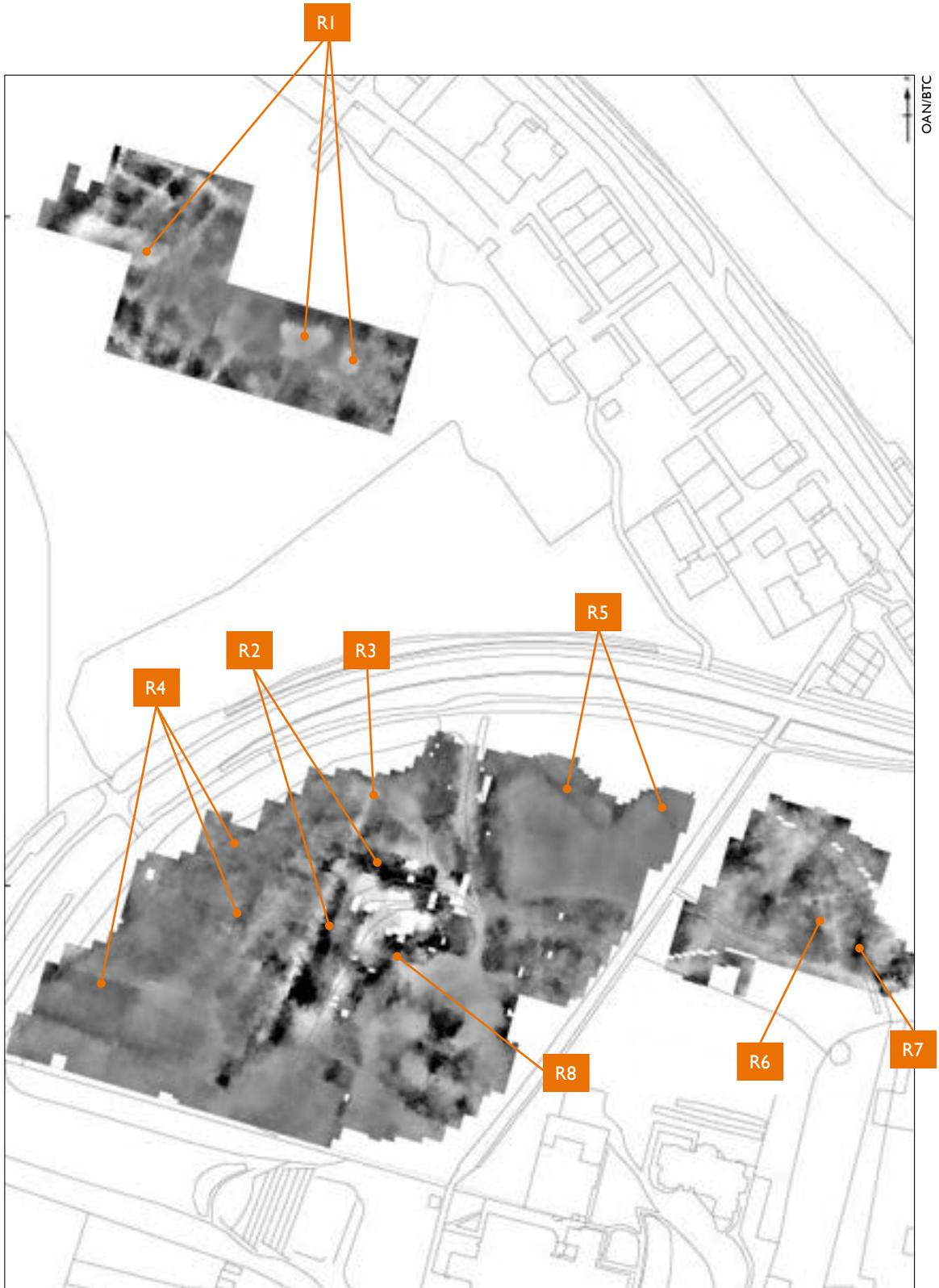
Resistance (Resistivity) survey of Vicarage Field West and East and Quay Meadow. For ease of reference the numbering of the anomalies follows that used in the OAN report with the addition of R8
