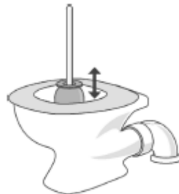
clearing a blocked WC
