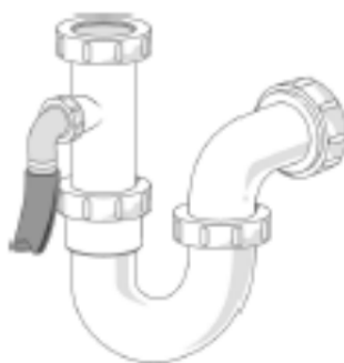
'p' trap with washing machine connection
