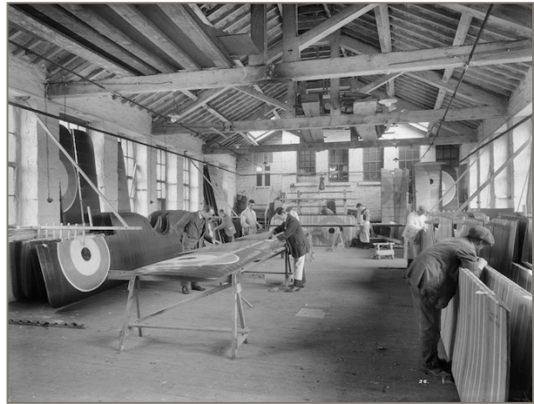
The production and inspection of bi-plane wings at Waring and Gillows, Lancaster, 1917 [Historic England ref. BL23741/036]
